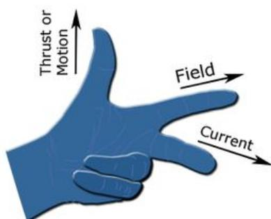
A **force** acts on a **current-carrying conductor** in a magnetic field. **Fleming's left-hand rule** shows the relative
