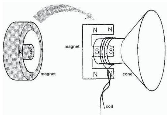
**Loud speakers** consist of a coil attached to a cone in a magnetic field. When **alternating current** flows through the coil, the cone is continuously pushed away and pulled back, making a **sound**. The **frequency** (and therefore pitch) of the sound can be altered by changing the frequency of the alternating current used.
